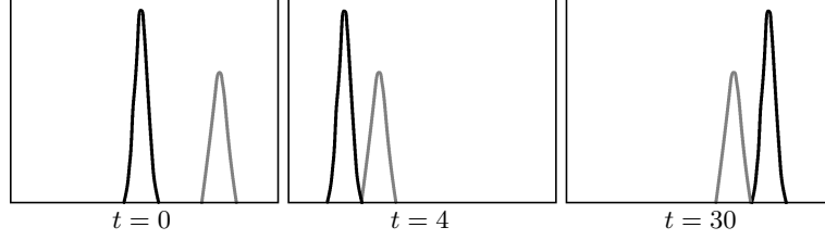
Figure 11. Snapshots of the soliton propagation obtained by simulating the process using a local parallel composition of two CA with local operators given by (57) and (59)
