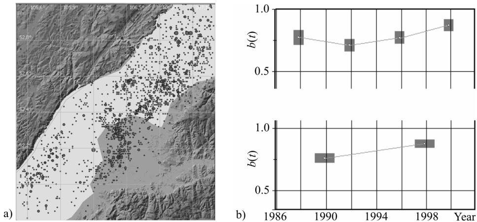
**Figure 11.** The BRZ area (a) shown in the frame in Figure 10 and changes in the profile of  $b$ -value parameter on 4-years (b, above) and 8-years intervals (b, below). The error of  $b$  definition is shown by segments and calculated by formula (1). The average  $b$  value grows from 0.75 up to 0.9
