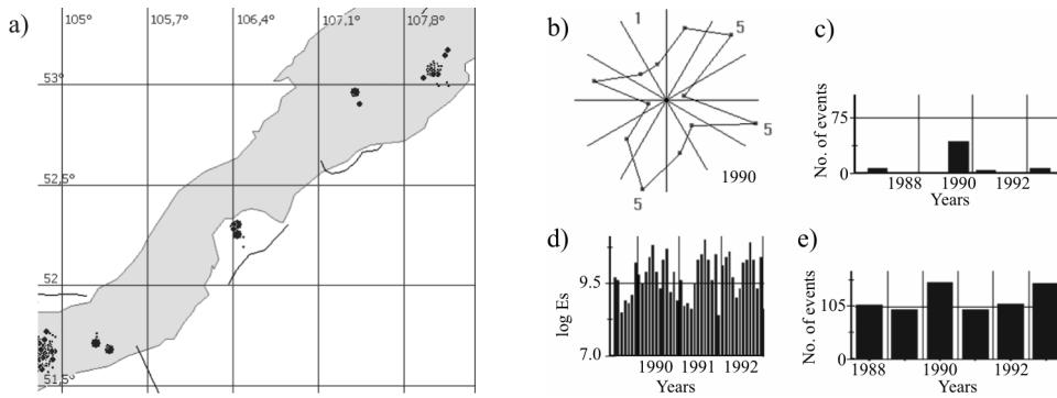
**Figure 9.** The nearest in time aftershocks: a) a map of the aftershocks sequences and swarms separated by the program for 1987–1992; b) a picture of azimuths distribution of the aftershocks pairs in 1990 when their number has appreciably increased; c) the number of events connected in aftershock sequences. The histograms describing the 1988–1992 seismic process ( $2 \leq M \leq 4$ ) after aftershocks separation: d) the total radiated energy per month and e) the number of events per year
