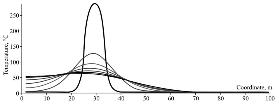
Figure 2. Thermal front of oil displacement at different instants time: 17 min, 4, 9, 13, 17, 21, 24 h
