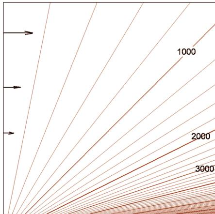
**Figure 5.** Tsunami wave front positions in the area with the parabolic bottom topography
