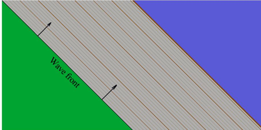
**Figure 4.** Sequential positions of the wave front when calculating the kinematics of the oblique front in an area with a constant depth. The zone of initial disturbance where  $t(i, j) = 0$  is colored by green
