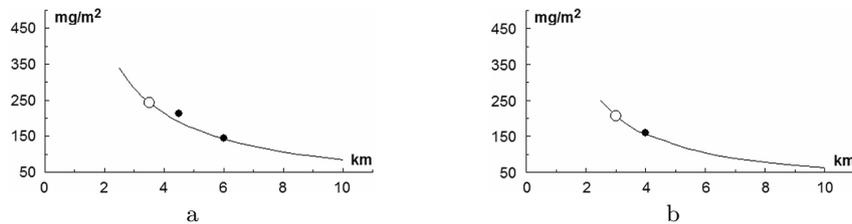
**Figure 2.** The dust deposition density from CHP-5 measured and recovered from dependence (5) in the direction to the east (a) and north-east (b):  $\circ$  reference points,  $\bullet$  reference observation points
