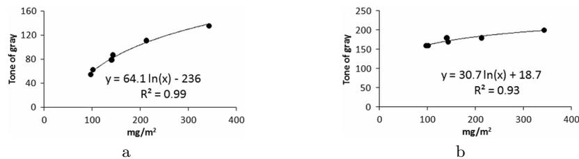
**Figure 4.** Functional relations between dust deposition from high-altitude pipes of Omsk CHP-5 at the observational points of the east direction and intensity of changes in gray tones in figures from 25.03.2010 (a) and 23.03.2015 (b)
